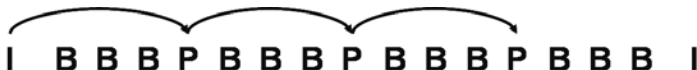
Fig. 3.1. Group of pictures and their encoding structure. The first picture of the group is an I frame, it is encoded using intra-prediction only. Differential coding is used to compress P frames and B frames. P frames are encoded after forming a motion-compensated prediction based on a preceding frame, as depicted by the prediction arrows. B frames are bi-directionally predicted frames, they depend on the neighboring P frames or I frames. This coding structure is periodically repeated to encode the entire video sequence.
