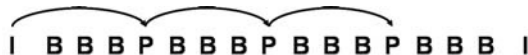
Fig. A.1. Encoding structure used for video streaming experiments with periodic I pictures. GOP length = 16
